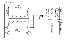
When the fan relay transformer is energized and the thermostat completes the connection from R to G the fan relay coil energizes. Line voltage power applied to contact common path travels to selected blower speed tap. Additional terminal Y and W are isolated tie point terminals to connect thermostat wiring to compressor and furnace (if required).
